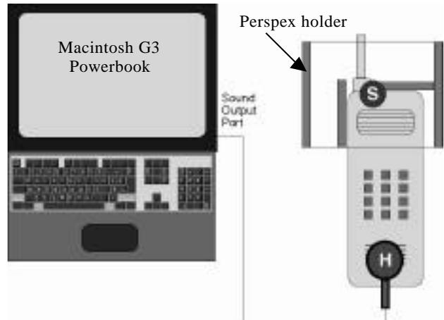
**Figure 2:** Schematic representation of the experimental setup. **S** is the position of the sample. **H** is the position of the headphone speaker.
