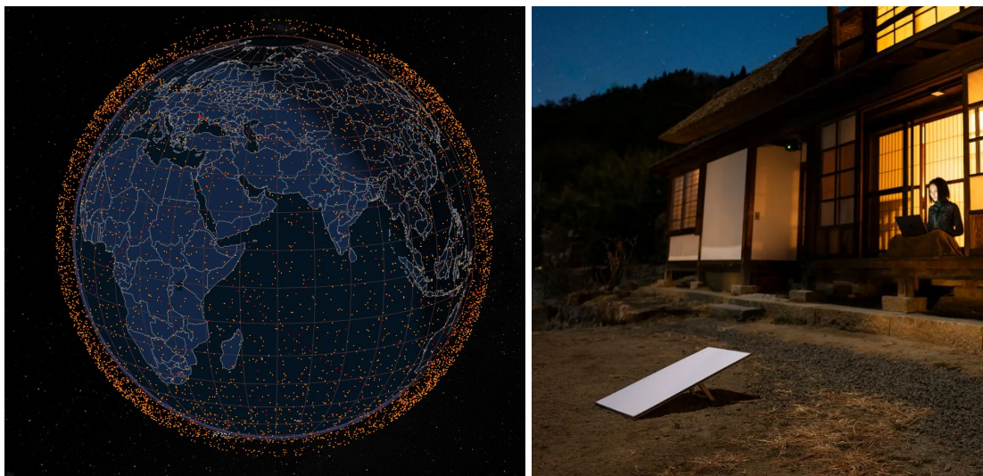
left: Visualization of active satellite constellations (satellitemap.space). As of Q4/2025, more than 14000 active satellites are in orbit, most of them being communication satellites in Low Earth Orbit (LEO); right: Starlink user terminal for satellite-based broadband internet access (starlink.com)
