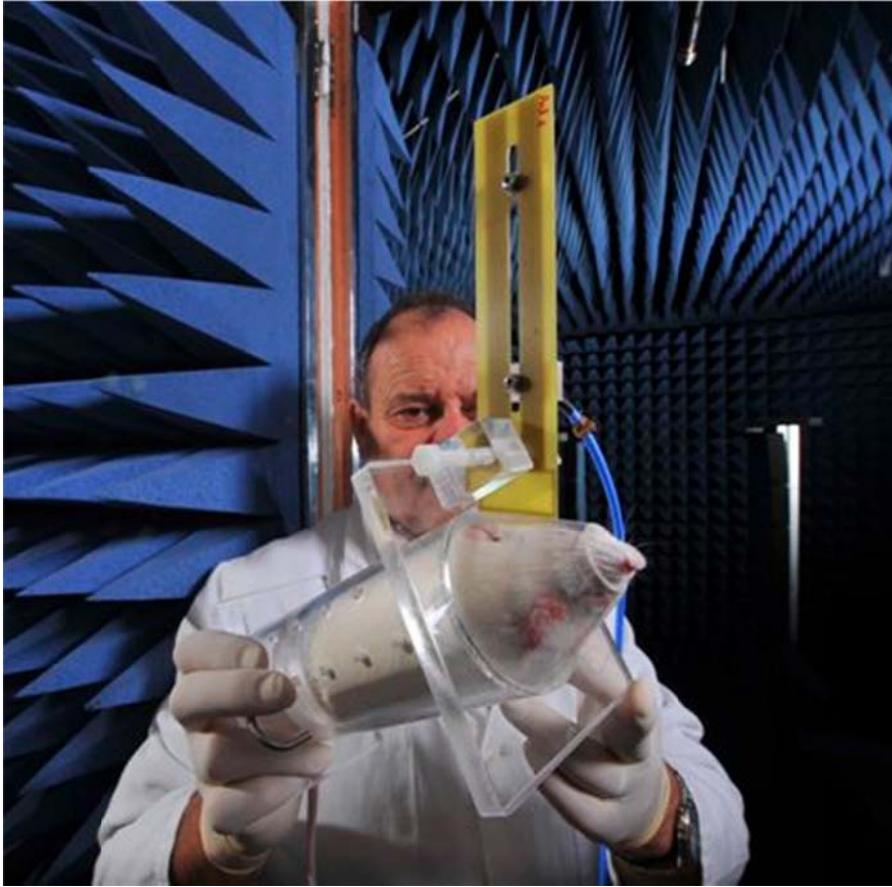
Figure : Head-only exposure set-up : a rat in a jig with the loop antenna
