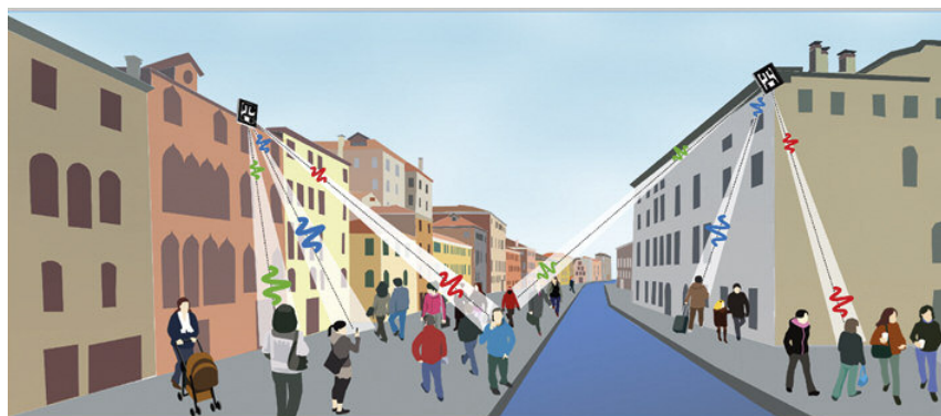
5G smart antennas deliver energy where it is needed rather than blanketing a large area. Illustration courtesy of Romain Bonjour, IEF, ETH Zurich.
